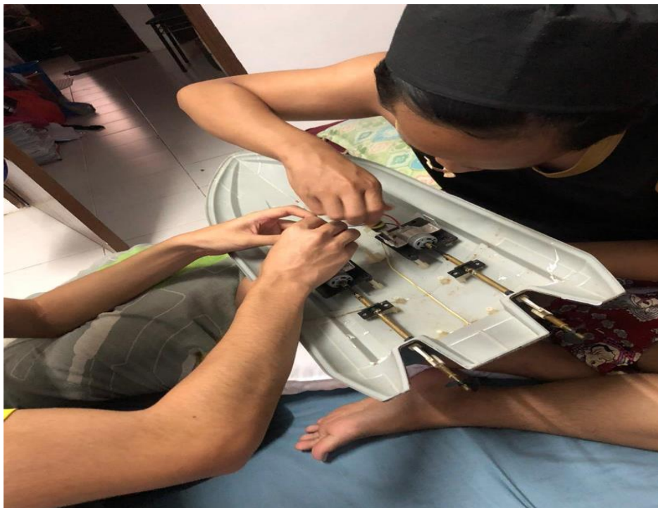
Figure 4.6 Testing the DC motor found inside of the boat
