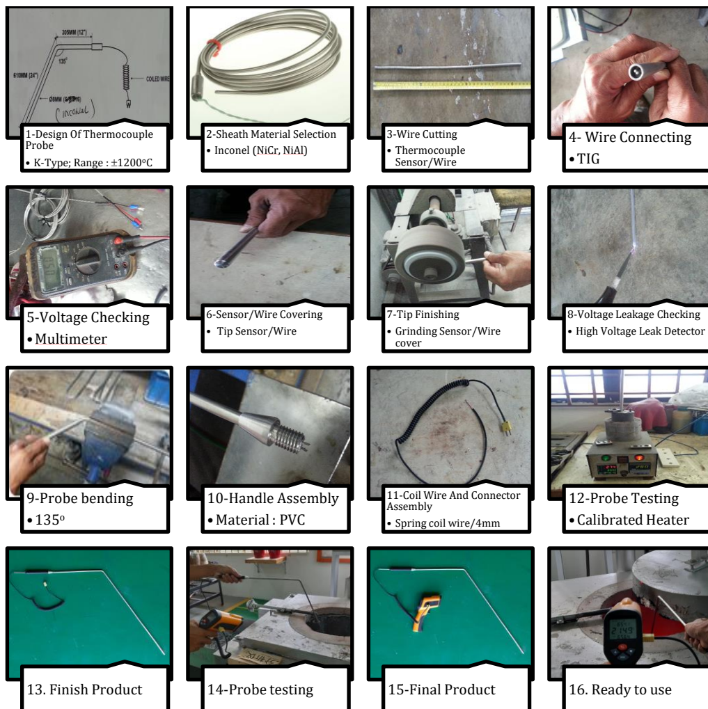
Figure 4: The Procedures for Fabrication Processes of the DIP.
